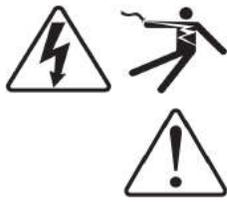
The addition of either symbol to a "Danger" or "Warning" safety label indicates that an electrical hazard exists which will result in personal injury if the instructions are not followed.
